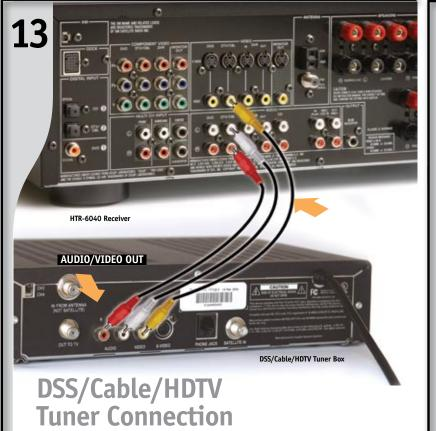
**Connect DSS/Cable/HDTV Tuner Box (optional)** Connect RCA audio/video cables (not included) and optional optical cable (not pictured) to "DTV/CBL" terminals on receiver to A/V OUT connections on Box as shown.
